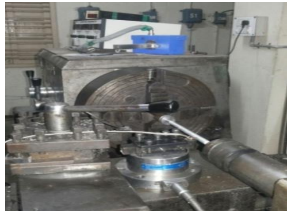
Figure 4: Cutting force measurement set-up
