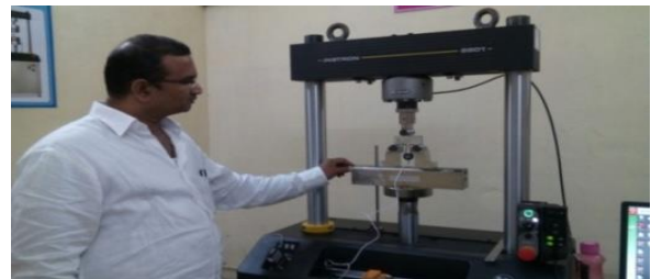
Figure 5: Fracture toughness experiment on 100 kN Instron Fatigue Testing Machine with SENB specimen
